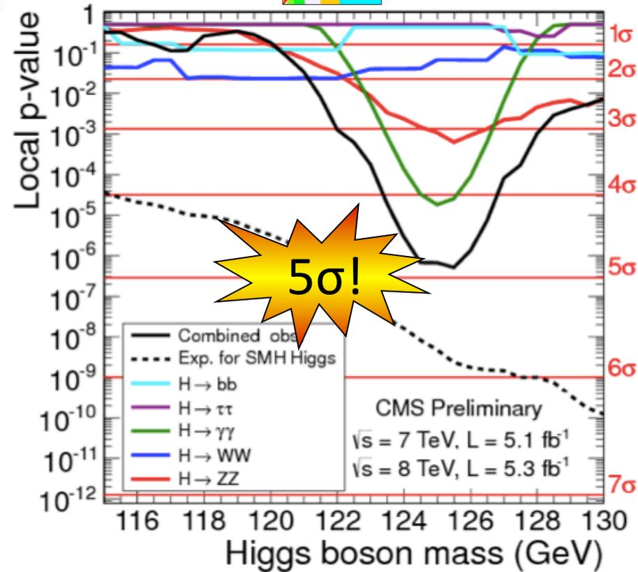
**Both experiments see an excess near 125 GeV! at  $\sim 5\sigma$
